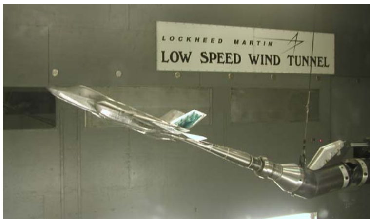
Figure 2. 1/12 th scale wind-tunnel model during buffet testing. (Courtesy of Lockheed-Martin Aeronautics)
